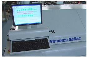
Figure 2: Digicom Electronics' soldering process provides temperature control in each zone.
