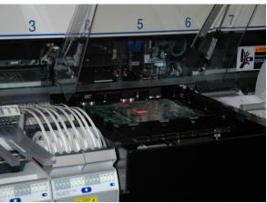
Figure 1: Digicom Electronics' capabilities include a pickand-place machine.
